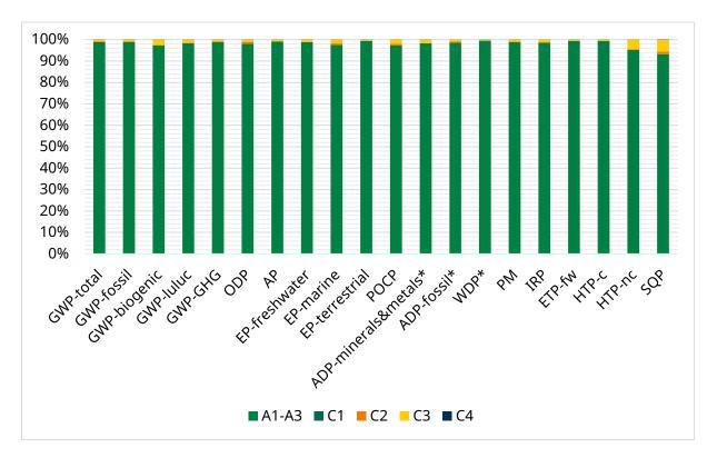
The dominating contributors to all environmental impacts are modules A1-A3. This is due to the use of steel as principal raw material which causes the main impact in all impact categories considered.
