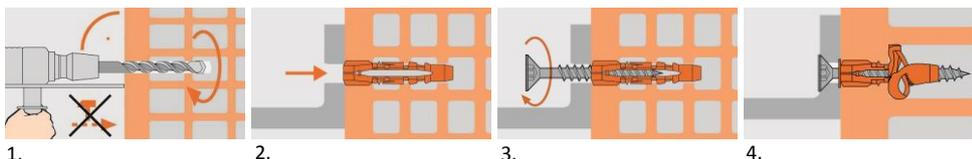
1. Make the drill hole with rotary drilling (no hammer drilling in hollow brick allowed),
