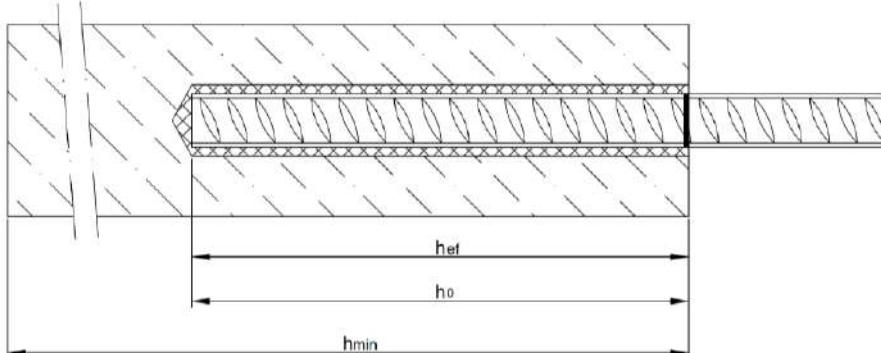
**Installation internal threaded rod IG-M6 to IG-M20**
