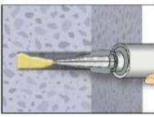
6. Starting from the bottom or back of the cleaned anchor hole, fill the hole up to approximately two-thirds with adhesive. Slowly withdraw the static mixing nozzle as the hole fills to avoid creating air pockets. For embedment larger than 190 mm an extension nozzle shall be used. Observe the gel-/ working times given in Table B5.
