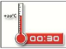
10. Allow the adhesive to cure to the specified time prior to applying any load or torque. Do not move or load the anchor until it is fully cured (attend Table B5).
