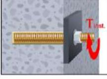
11. After full curing, the add-on part can be installed with up to the max. torque (Table B1 or B3) by using a calibrated torque wrench.
