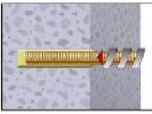
8. Push the threaded rod or reinforcing bar into the anchor hole while turning slightly to ensure positive distribution of the adhesive until the embedment depth is reached.
