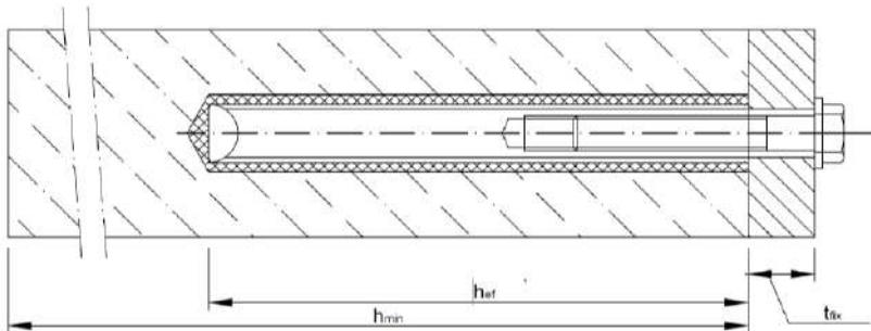
$t_{\text{fix}}$  = thickness of fixture $h_{\text{ef}}$  = effective anchorage depth $h_0$  = depth of drill hole $h_{\text{min}}$  = minimum thickness of member**Mungo Injection system MIT-Hybrid for concrete**
