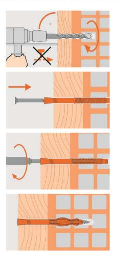
Drill the hole according to the method given in Table C6 and C7 by **rotary drilling** (without hammering) or **hammer drilling**.
