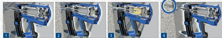
Press the tool against the fixture and base material. Wait a fraction of a second to let the gas and air create an ignitable mixture. Press the trigger to perform the fixing to the steel or concrete. Remove your finger from the trigger and retract the tool from the fixing point.
