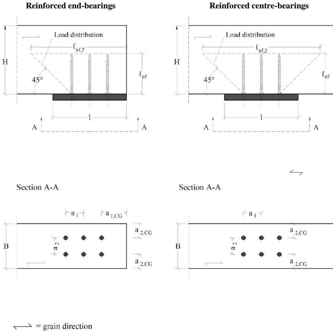
The design load-carrying capacity for a reinforced contact area with screws with a full thread or threaded rods at an angle  $\alpha$  to the grain of  $45^\circ < \alpha < 90^\circ$  shall be calculated from:
