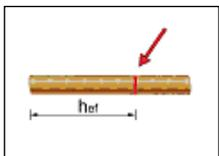
4. Prior to inserting the anchor rod into the filled bore hole, the position of the embedment depth shall be marked on the anchor rods.
