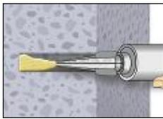
6. Starting from the bottom or back of the cleaned anchor hole fill the hole up to approximately two-thirds with adhesive. Slowly withdraw the static mixing nozzle as the hole fills to avoid creating air pockets. For embedment larger than 190 mm an extension nozzle shall be used. Observe the gel-/ working times given in Table B3.
