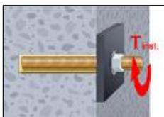
10. After full curing, the add-on part can be installed with the max. torque (Table B1) by using a calibrated torque wrench.
