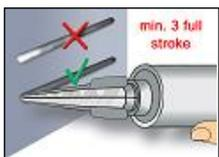
5. Prior to dispensing into the drill hole, squeeze out separately a minimum of three full strokes and discard non-uniformly mixed adhesive components until the mortar shows a consistent grey colour. For foil tube cartridges it must be discarded a minimum of six full strokes.
