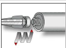
3. Attach a supplied static-mixing nozzle to the cartridge and load the cartridge into the correct dispensing tool. Cut off the foil tube clip before use. For every working interruption longer than the recommended working time (Table B3) as well as for new cartridges, a new static-mixer shall be used.
