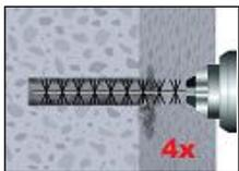
2b Check brush diameter (Table B2) and attach the brush to a drilling machine or a battery screwdriver. Brush the hole with an appropriate sized wire brush  $> d_{b,min}$  (Table B2) a minimum of four times. If the bore hole ground is not reached with the brush, a brush extension shall be used (Table B2).
