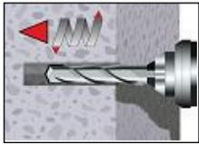
1 Drill with hammer drill a hole into the base material to the size and embedment depth required by the selected anchor (Table B1). In case of aborted drill hole: the drill hole shall be filled with mortar.
