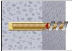
7. Push the threaded rod into the anchor hole while turning slightly to ensure positive distribution of the adhesive until the embedment depth is reached.
