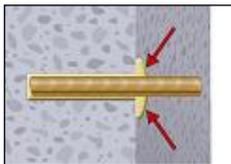
8. Be sure that the anchor is fully seated at the bottom of the hole and that excess mortar is visible at the top of the hole. If these requirements are not maintained, the application has to be renewed. For overhead application the anchor rod should be fixed (e.g. wedges).
