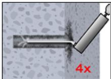
2c Finally blow the hole clean again with compressed air (min. 6 bar) or a hand pump (Annex B2) a minimum of four times. If the bore hole ground is not reached an extension shall be used.
