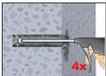
**After cleaning, the bore hole has to be protected against re-contamination in an appropriate way, until dispensing the mortar in the bore hole. If necessary, the cleaning repeated has to be directly before dispensing the mortar. In-flowing water must not contaminate the bore hole again**
